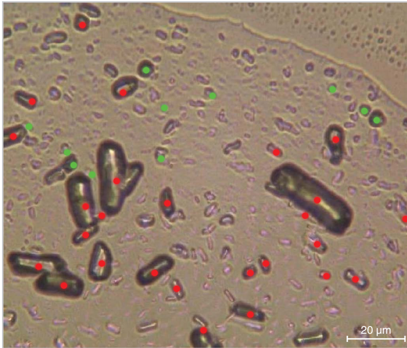
Discrete points map; fast, targeted analysis of single particles within a nasal spray droplet. The image reveals the drug and excipient location relative to the white light image.
