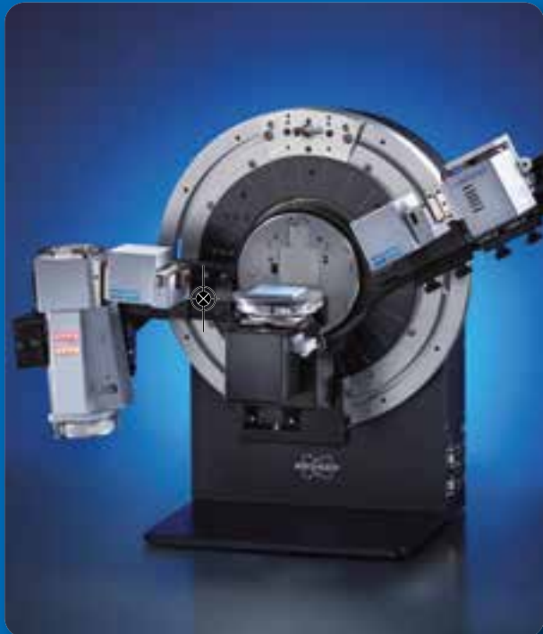
Grazing Incidence Diffraction TWIN/TWIN setup
