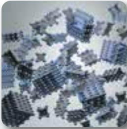
Randomly oriented crystallites
