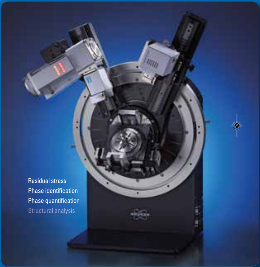
Texture or stress measurements in side-inclination (psi) mode
