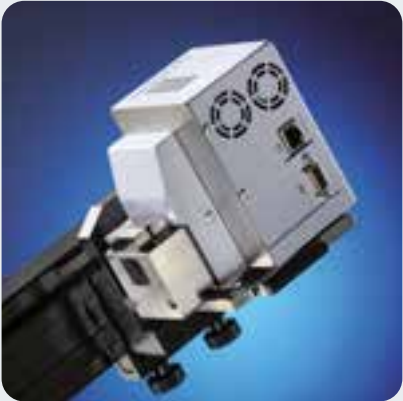
LYNXEYE XE-T in 90° mode for 2-D measurements
