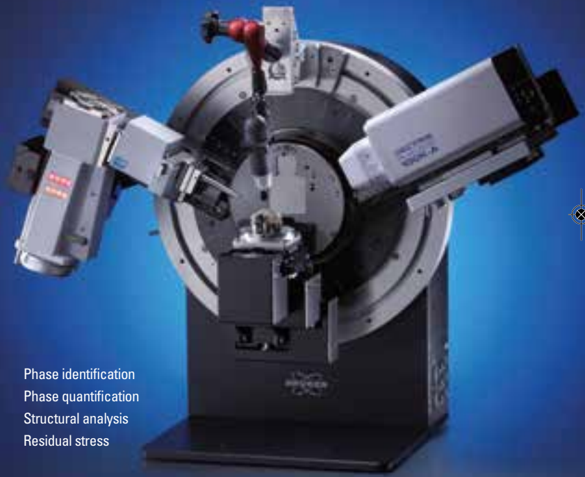
μXRD measurement with PILATUS3 R 100K-A
