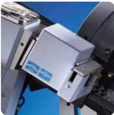
Push-button switch of optics -TWIN
