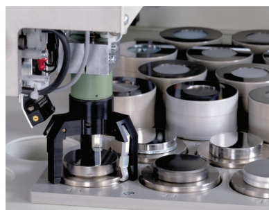
A metal control sample is loaded to verify the instrument performance (ARL 9900 XRF version)
