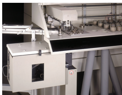
Automatic labeling of a metal sample on the reverse side before analysis (ARL 9900 XRF version)
