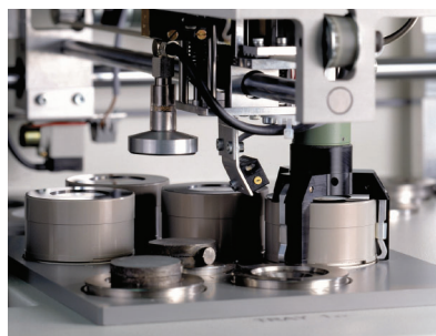
Loading of a cassette for analysis using the gripper (ARL 9900 XRF version)
