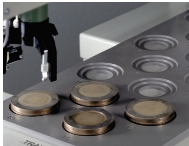
Loading of a pellet sample using the gripper (ARL 9900 XRF version)
