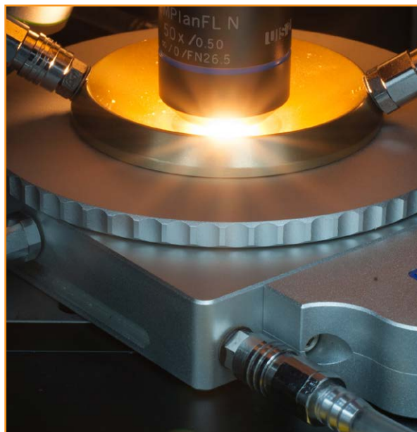
Using LiveTrack to maintain focus on the surface of a sample in a high temperature cell.
