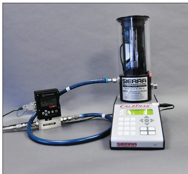
CalTrak MFM/MFC Calibration Setup
