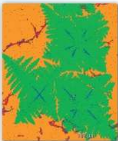
Raman imaging can be used to evaluate the quality of materials such as graphene films and provide essential feedback for development of production methods. This image shows the structural composition of a graphene film using Raman imaging and comprises over 170,000 spectra in a 188 \times 227 micron area.
