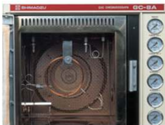
Fig. 7 Quartz Capillary Column Mounted with CLH-800
