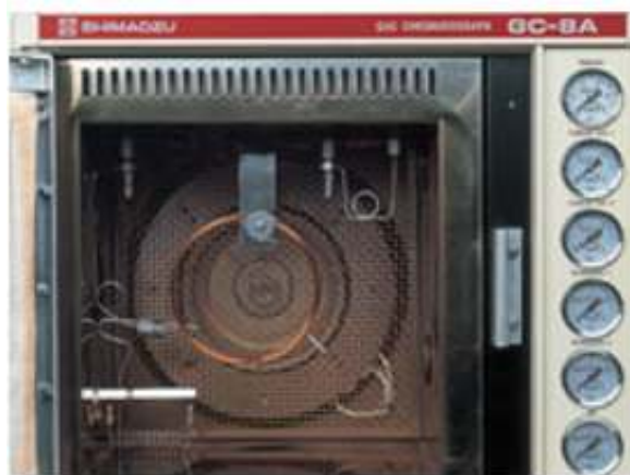
Fig. 7 Quartz Capillary Column Mounted with CLH-800
