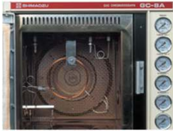
Fig. 7 Quartz Capillary Column Mounted with CLH-800
