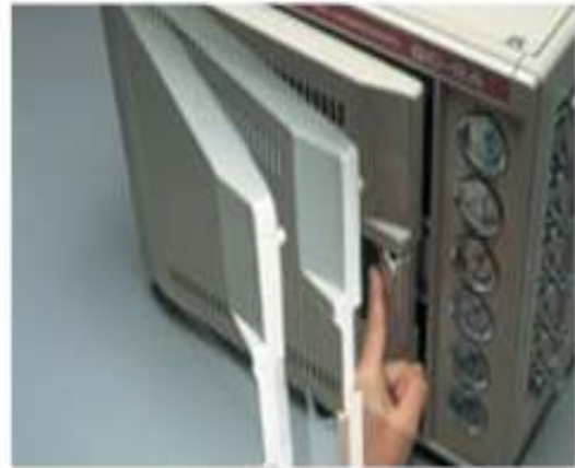
Fig. 3 Operation of Column Oven Door
