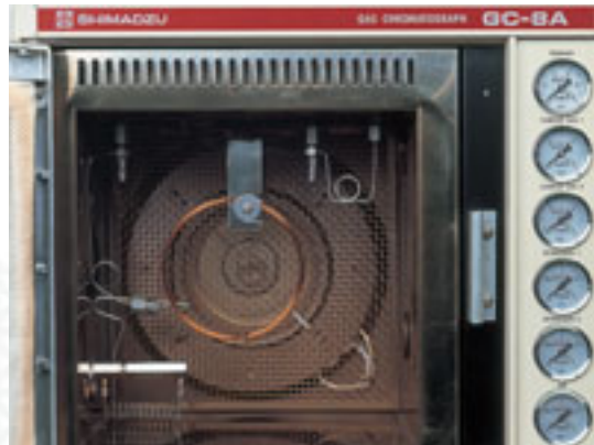
Fig. 7 Quartz Capillary Column Mounted with CLH-800
