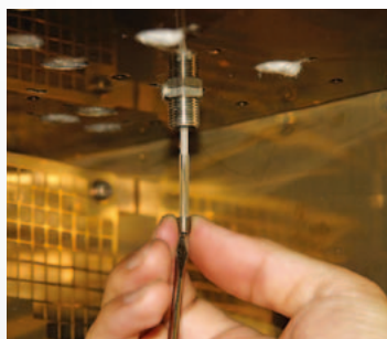
Simple nozzle replacement supports both capillary and packed columns.
