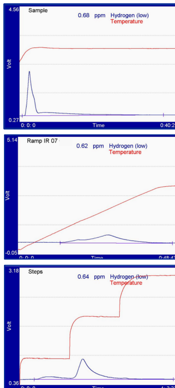
Figure 7: Steel sample analyzed with isothermal conditions (upper), temperature ramping (middle) and temperature gradients (lower) as a function of time. Note: Red profile indicates temperature and blue profile indicates hydrogen response.
