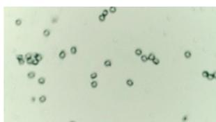
Sample : 10  $\mu\text{m}$  diameter polystyrene bead on BaF<sub>2</sub> window plate
