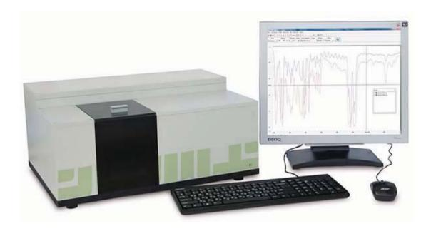
Multipurpose laboratory IR Fourier-spectrometers IROS P01 and IROS P02 are designed for routine measurements and scientific researches in the mid-infrared range.
