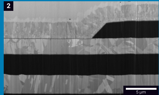
Fig. 2: High material contrast of under-bump metal layers observed at 1 keV with the E-T detector
