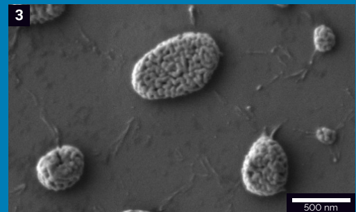
Fig. 3: Characterization of Au nanoparticle on Si/SiO 2 substrate. The nanoporous structure, size and surface morphology of these nanoparticles can be investigated. Sample imaged at 500 eV with the E-T detector.
