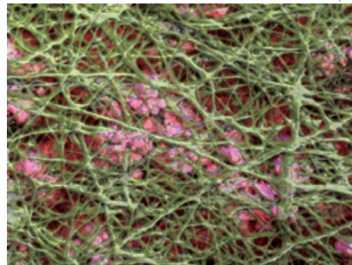
Specimen: Egg-shell membrane Accelerating voltage: 10 kV, Magnification: \times 500 Low-vacuum mode Top: Backscattered electron stereoscopic image Bottom: Composite elemental map (Green: C, Blue: O, Red: Ca)
