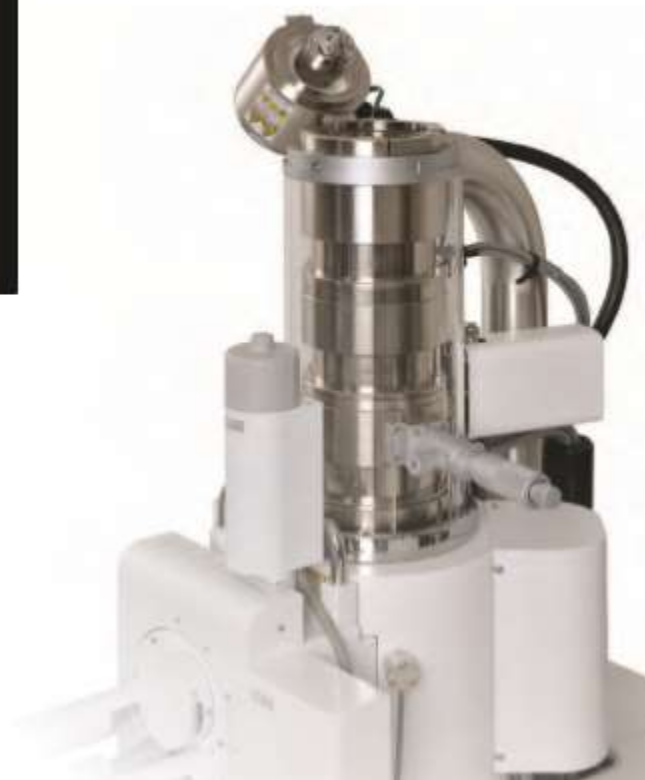
Filaments are pre-centered for easy replacement.
