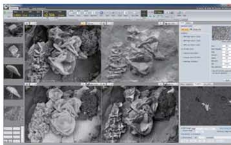
Quadruple image (640 x 480 pixels x 4) Real time 4 different image display for effective multiple image comparison, for example, SE image, BSE compositional image, BSE topographic image, and BSE 3D image.
