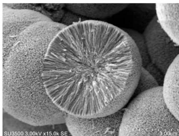
Sample : Titanium Oxide Particle, Accelerating Voltage : 3 kV, Magnification : x 15,000, Signal : Secondary Electron (SE), Without metal coating Sample courtesy : Prof. Masato Kakihana Tohoku University
