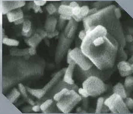
Sample: ZnO, Accelerating Voltage: 5 kV Magnification: 150,000x Signal: Secondary Electron (SE) Without metal coating
