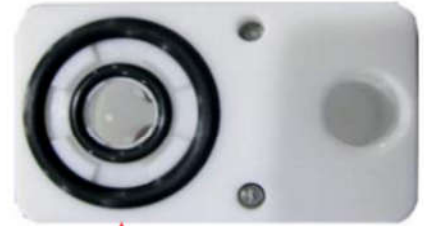
Active area will be determined by O-ring's position.
