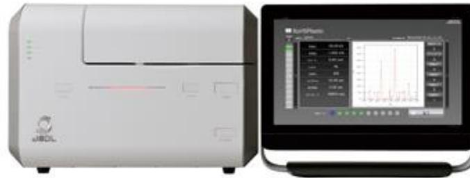
The JSX-1000S is an X-ray fluorescence spectrometer that provides quick, easy elemental analysis using touch screen operation. It is equipped with functions for conventional qualitative and quantitative analysis (FP method, calibration curve method), as well as screening for RoHS elements. With a variety of both hardware and software options available, it is customizable to cover a wide range of analysis needs.
