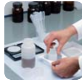
■ Cover bottom of liquid cup with transparent film
