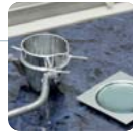
■ Casting mold with finished glass bead
