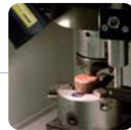
■ Check sample height at molding cutter
