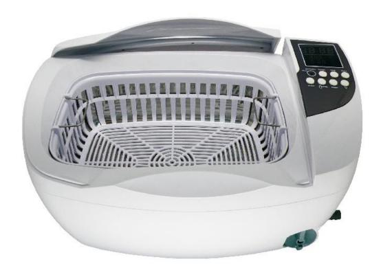
Ultrasonic cleaners function by producing sound waves that are transmitted into the tank and cleaning solution. These waves create millions of microscopic bubbles, which collapse or 'implode', releasing large amounts of energy, which scrub the surface clean. This process is called 'Cavitation'.
