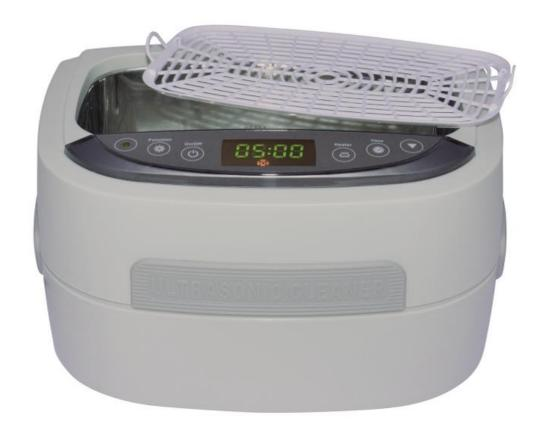
Ultrasonic cleaners function by producing sound waves that are transmitted into the tank and cleaning solution. These waves create millions of microscopic bubbles, which collapse or 'implode', releasing large amounts of energy, which scrub the surface clean. This process is called 'Cavitation'.
