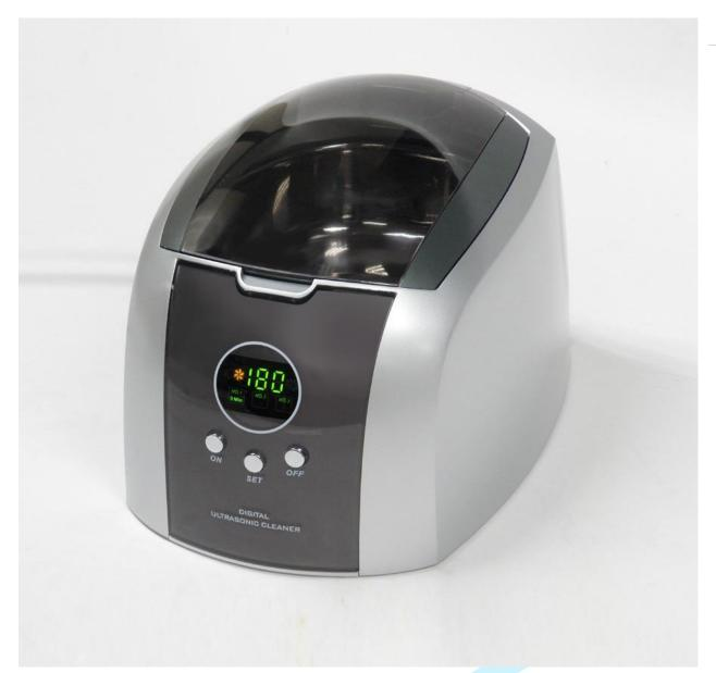
Ultrasonic cleaners function by producing sound waves that are transmitted into the tank and cleaning solution. These waves create millions of microscopic bubbles, which collapse or 'implode', releasing large amounts of energy, which scrub the surface clean. This process is called 'Cavitation'. These tiny bubbles create incredible cleaning results not only to the surface, but by penetrating the fner detail and recesses in jewellery and small items to restore them to their former glory.
