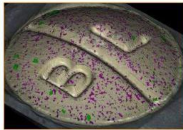
Allergy relief tablet showing low concentration API (green) and maize starch (magenta).
