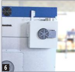
6 Air cooling extractor
