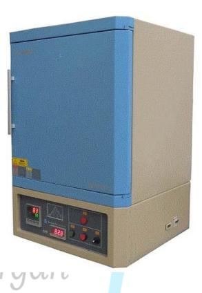
KSL-1200X-L5-UL is a five sides heating muffle furnace, which is designed for annealing superalloy and precious metal with more uniform temperature zone and SiC sheet is installed on the bottom of the chamber which can load heavy sample up to 100 kg.
