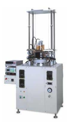
Applying a 500°C maximum temperature difference across a thermoelectric module under test, the PEM-2 finds the thermoelectric conversion rate h by finding the generated power P when a one-dimensional heat flow Q passes through the module. A single run generates a complete set of data characterizing module performance over a wide range of temperatures, and shows the results automatically in a set of elegant graphical displays.
