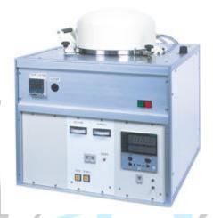
Measures specific heat capacity, latent heat, transformation points
