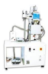
Temperature dependency measurements of insulator samples
