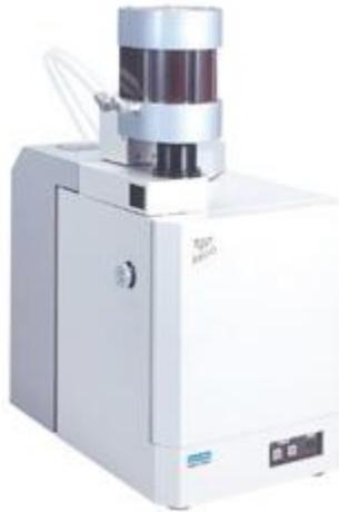
Unique signal TG and separate DTA measurements
