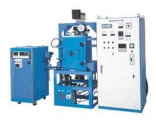
Thermal diffusivity measurements in ultra-high temperature regions up to 3000  $^{\circ}\text{C}$  maximum
