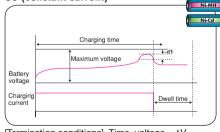
[Termination conditions] Time, voltage, – $\Delta V\!\!,$  temperature, and  $\Delta T/\Delta t$
